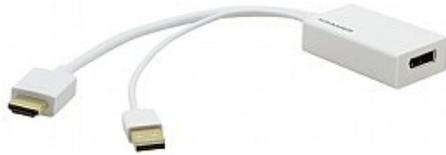
ADC-HM/DPF is a perfect solution for connecting devices with HDMI outputs to a DisplayPort monitor or projector. The adapter cable supports resolutions up to 4K@30Hz, is HDCP 2.0 compliant and provides quick and easy, plug-and-play installation with no software or drivers to install. The auxiliary USB connector enables power supply through a USB-A port when the power from the HDMI source is not sufficient
